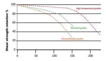
Above: Graph showing how temperature affects strength retention of Permabond anaerobic adhesives.
