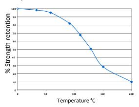
UV7141 can withstand higher temperatures for brief periods (such as for paint baking and wave soldering processes) providing the joint is not unduly stressed. The minimum temperature the cured adhesive can be exposed to is -55°C (-67°F) depending on the materials being bonded.
