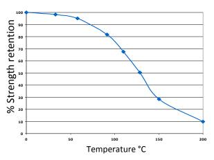
UV640 can withstand higher temperatures for brief periods (such as for paint baking and wave soldering processes) providing the joint is not unduly stressed. The minimum temperature the cured adhesive can be exposed to is -55°C (-67°F) depending on the materials being bonded.
