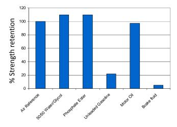
Specimens were immersed for 30 days at 85 $^{\circ}$ C and tested at room temperature.
