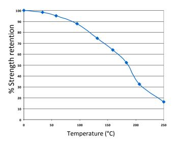
TA437 can withstand higher temperatures for brief periods (such as for paint baking and wave soldering processes) providing the joint is not unduly stressed. The minimum temperature the cured adhesive can be exposed to is -55°C (-65°F) depending on the materials being bonded.
