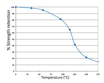
TA436 can withstand higher temperatures for brief periods (such as for paint baking and wave soldering processes) providing the joint is not unduly stressed. The minimum temperature the cured adhesive can be exposed to is -55°C (-65°F) depending on the materials being bonded.
