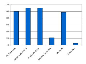
Specimens were immersed for 30 days at 85°C and tested at room temperature.
