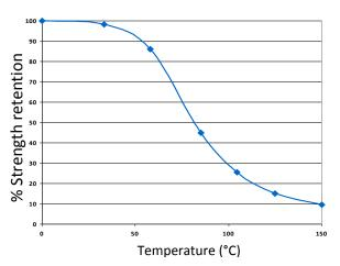
MT3809 can withstand higher temperatures for brief periods (such as for paint baking and wave soldering processes) providing the joint is not unduly stressed. The minimum temperature the cured adhesive can be exposed to is -40°C (-40°F) depending on the materials being bonded.
