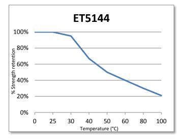
ET5144 can withstand higher temperatures for brief periods (such as for paint baking and wave soldering processes) providing the joint is not unduly stressed. The minimum temperature the cured adhesive can be exposed to is -40°C (-40°F) depending on the materials being bonded.
